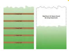
losing more than 1 metre of valuable airspace each week to daily cover material. For a landfill with a daily work face of around 500m<sup>2</sup>, this equates to a staggering 500 cubic metres of airspace wasted each week!
