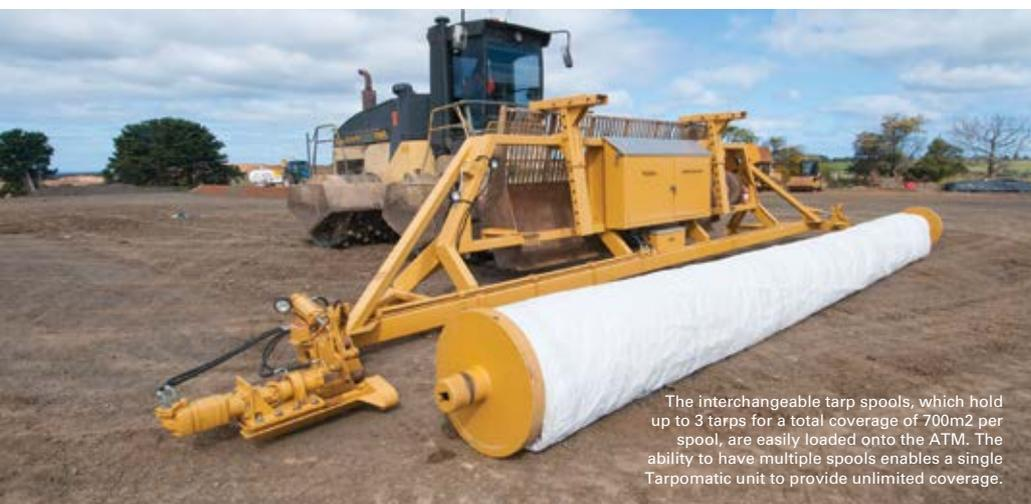
The interchangeable tarp spools, which hold up to 3 tarps for a total coverage of 700m<sup>2</sup> per spool, are easily loaded onto the ATM. The ability to have multiple spools enables a single Tarpomatic unit to provide unlimited coverage.
